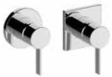
59551 Single lever mixer DN 15 Mixing cartridge with ceramic sealing gaskets, temperature controlled, set complete with: handle, sleeve, rosette (round or square) and installation unit, suitable for rough part no. 59551/000070
